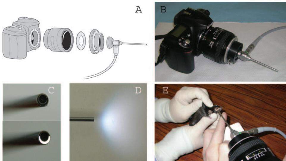
**FIGURE 1.** (A, B) Scheme and general view of the TEFI system. (C) Tip of the endoscope showing the crescent-shaped illumination. (D) Dispersion of light at the tip. Note the chromatic aberration revealed by the blue-green halo. (E) TEFI procedure.
